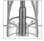
In this cutaway view the precious fluids well is visible. Total volume in this chamber is less than one milliliter. Since it is continuously fillable, there is minimal waste of precious fluids.
