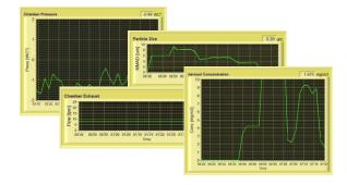
The SPM is designed to acquire data selectively from the LabFlow V II control unit and monitoring devices used in conjunction with our inhalation systems. The SPM is the perfect tool for users that require GLP compliance for their inhalation systems.
